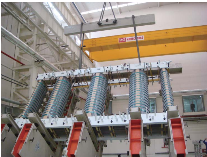
• Tilting platform for iron core
