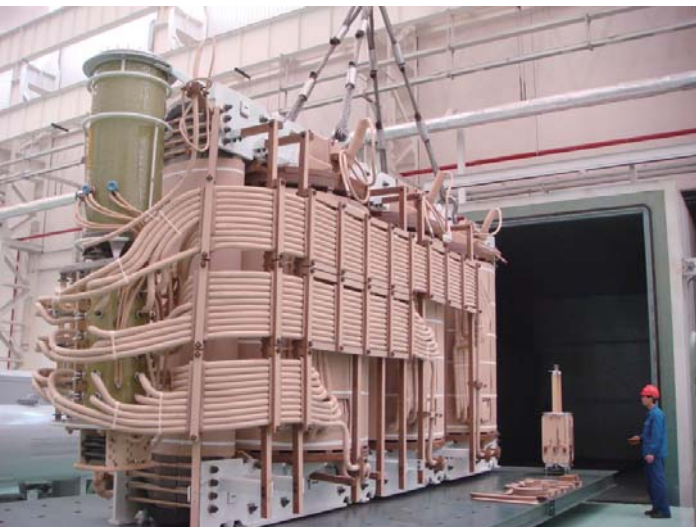
• Vapor-phase drying (VPD) Process (Active parts drying)
