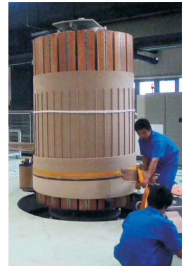
• Winding under production
