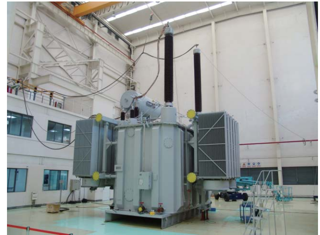
• 500kV transformer under testing
