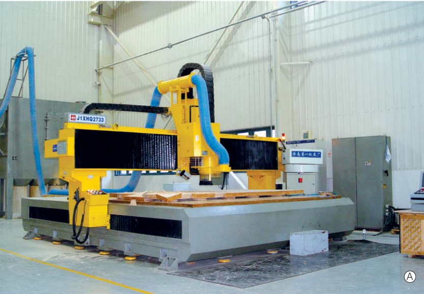
• (A) (B) Digital processing center for insulation parts
