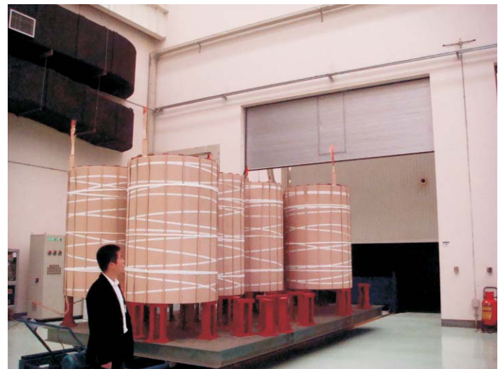
• Vapor-phase drying (VPD) Process(Oil drying)
