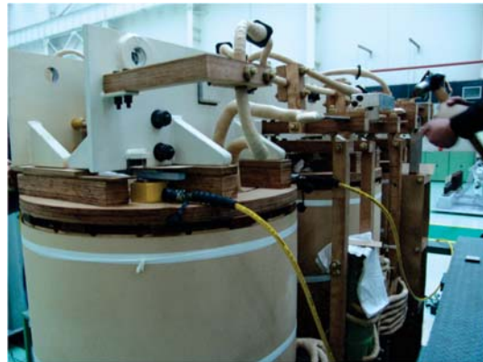
• Transformer body compressing device with synchronized control
