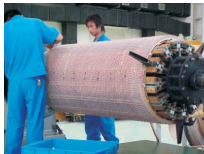
• Winding made of transposed conductor
