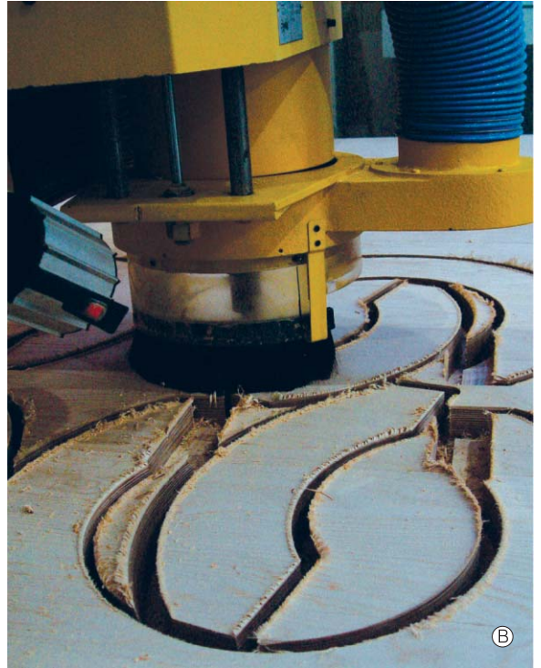
• (A) (B) Digital processing center for insulation parts
